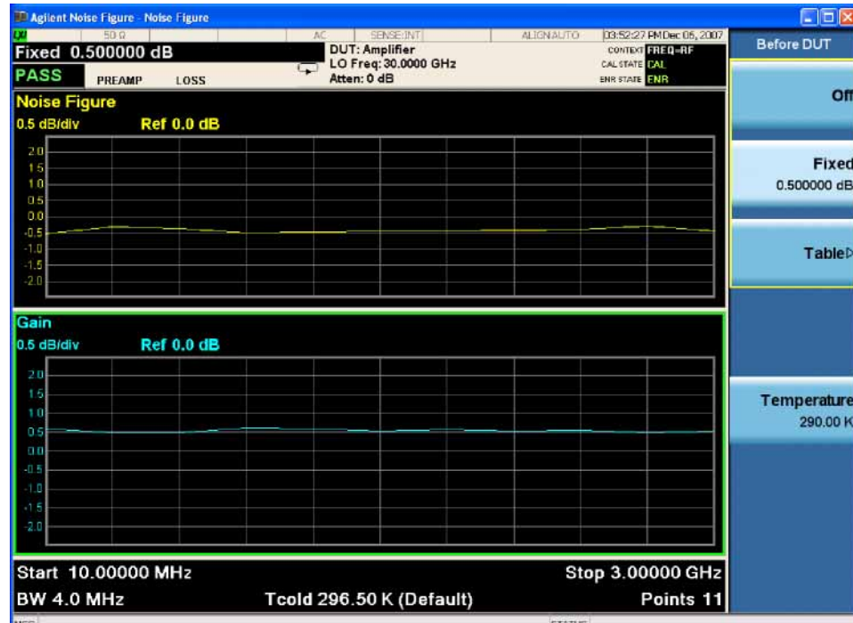
Figure 2-38 Fixed Loss Compensation
