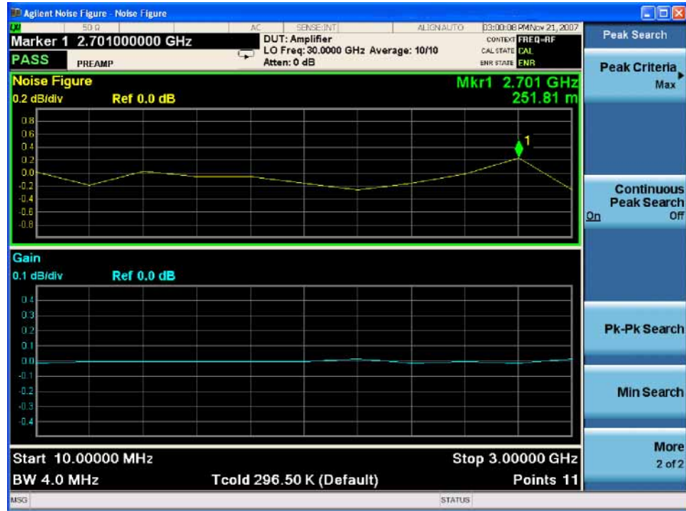
Figure 2-12 Typical Trace Showing Maximum Point Found
